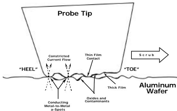
Figure 1 - Probe tip and aluminum contact pad interface.
